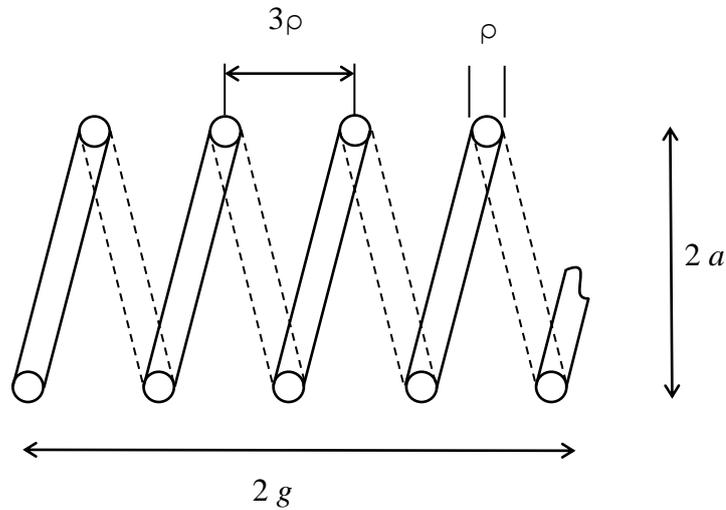
Figure 4. Coil winding geometry.
