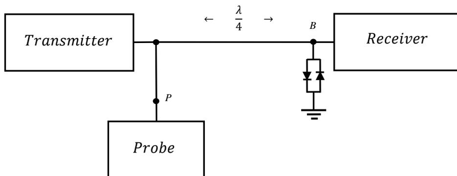
Figure 1. Block diagram of the NMR spectrometer.
