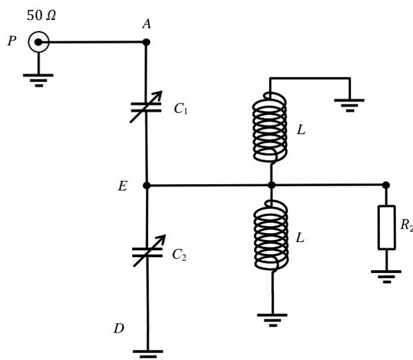
**Figure 5.** Equivalent circuit during the rf pulse.
