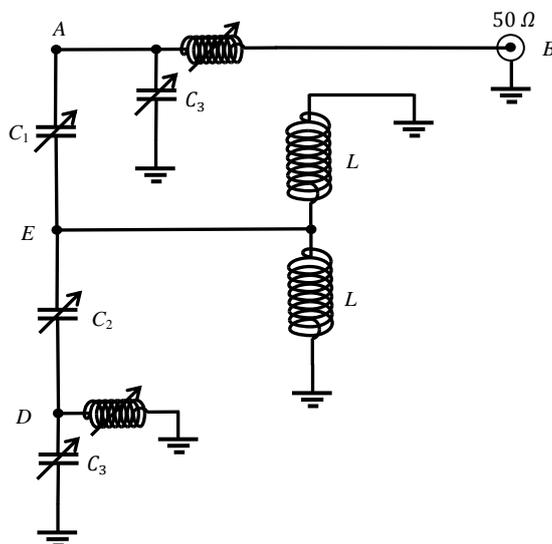
Figure 6. Equivalent circuit during the signal reception.
