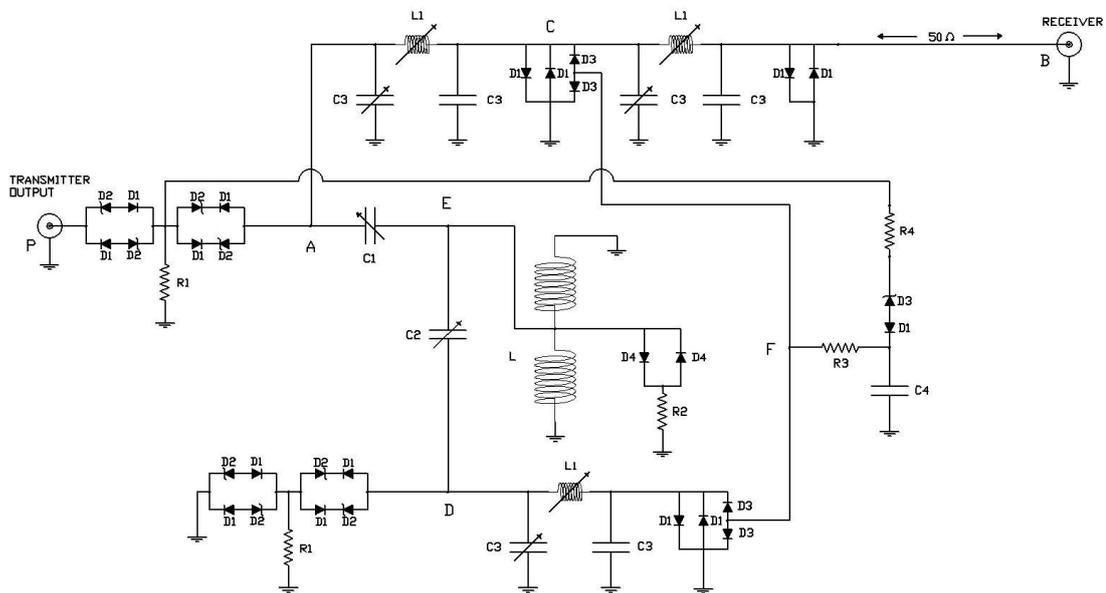
**Figure 3.** Probe circuit.  $R_1 = 1 k\Omega$ ,  $R_2 = 900 \Omega$ ,  $R_3 = 1 k\Omega$ ,  $R_4 = 200 \Omega$ ,  $C_1 \approx 40 pF$ ,  $C_2 \approx 1490 pF$ ,  $C_3 = 1.6 \mu F$ ,  $D_1 = 1N41448$ ,  $D_2 = 1N5342B$  6.8V Zener,  $D_3 = 1N5347B$  10V Zener.
