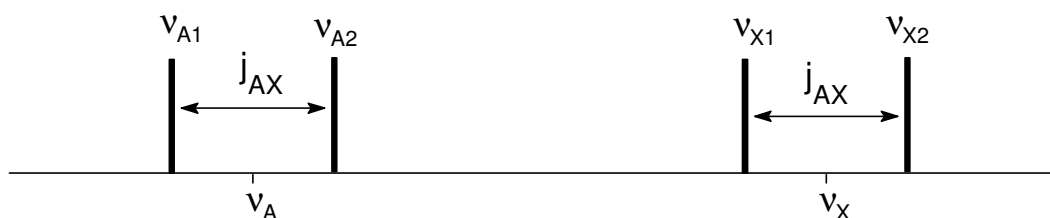
Figure 4. Spectrum of a coupled system formed by nuclei A and X with spin \frac{1}{2}
