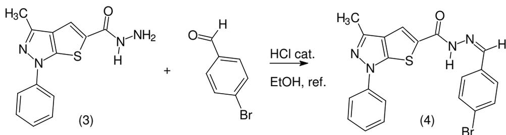
**Figure 2.** Scheme for preparation of (4'-bromo-benzylidene)-3-methyl-1-phenyl-1*H*-thieno[2,3c]pyrazolo-5-acyl hydrazone (compound 4).
