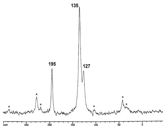
**Figure 4.** Solid-state  $^{13}\text{C}$  CP/MAS spectrum of p-bromobenzaldehyde. (\*) denotes spinning sidebands
