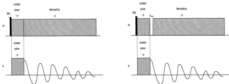
**Figure 3.** Cross-polarization pulse sequences, without (left) and with (right) interrupted decoupling, used for dipolar dephasing experiments (adapted from ref. 6).
