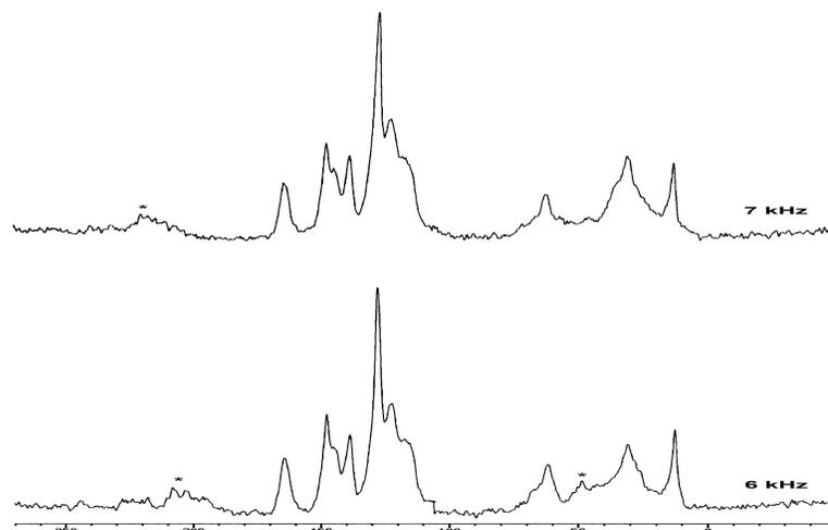
**Figure 5.** Solid-state  $^{13}\text{C}$  CPMAS spectrum of acylhydrazide (3), at spinning rate of 6 kHz (bottom) and 7 kHz (top). (\*) denotes spinning sidebands
