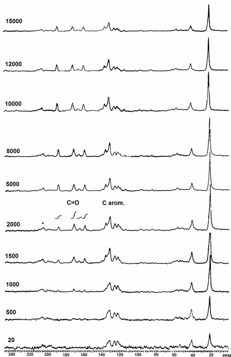
Figure 7. Solid state  $^{13}\text{C}$  CPMAS spectra obtained with variation in contact time ( $\mu\text{s}$ ) for compound 2.
