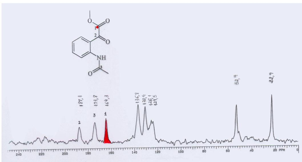
Figure 5.  $^{13}\text{C}$  CPMAS solid state NMR spectrum obtained for compound 1.
