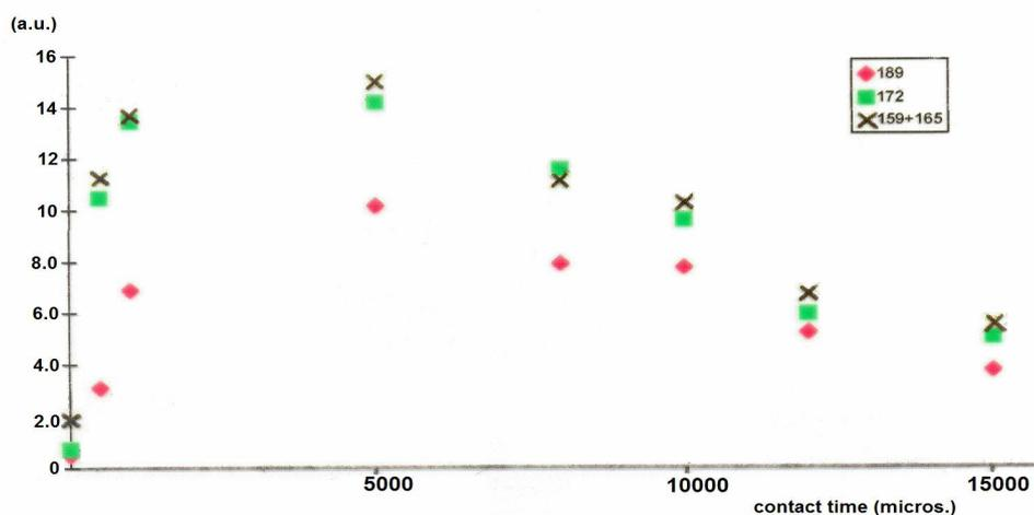
**Figure 10.** Variation in the intensity signal (arbitrary unities) in function of contact time (in  $\mu\text{s}$ ), obtained for compound **2**; the areas of the signals at 160 and 166 ppm (S-cis and S-trans) were added.
